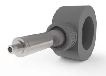
Litre Meter started manufacturing the Pelton Wheel turbine in 1975. These usually had some stainless steel components together with a plastic rotor, elastomer seals and sapphire bearings. All plastic versions soon followed, including all Polypropylene, all PFA, all PVC and all PVDF. The other wetted parts are still sapphire with a suitable elastomer such as FKM or FFKM for the single O ring seal.
